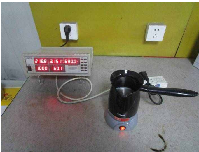
Power Consumption test with 220V
