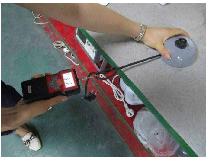
Power cord pull test
