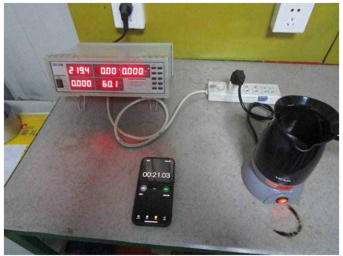
Boil-DRY protection test
