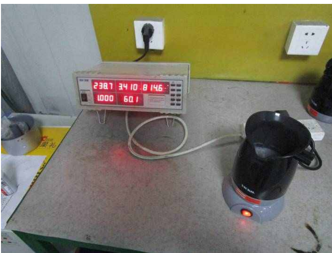
Power Consumption test with 240V
