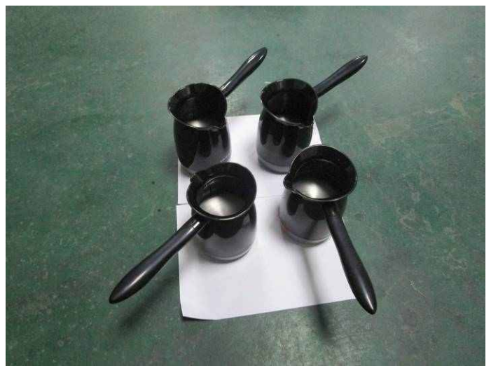
Water leakage check
