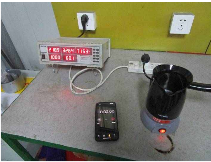
Boil-DRY protection test
