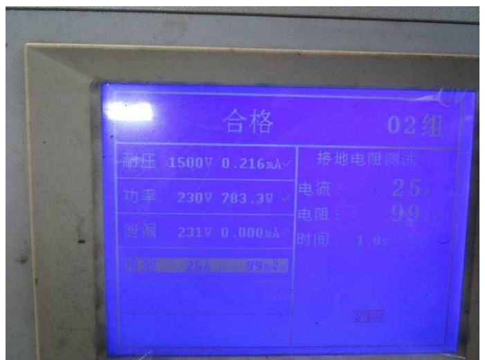
Hi-pot and Earth continuity test
