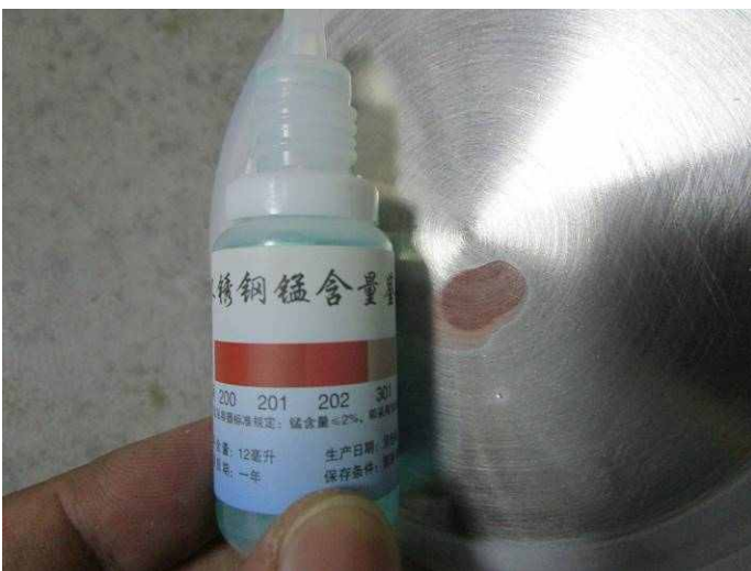
Stainless Steel material test
