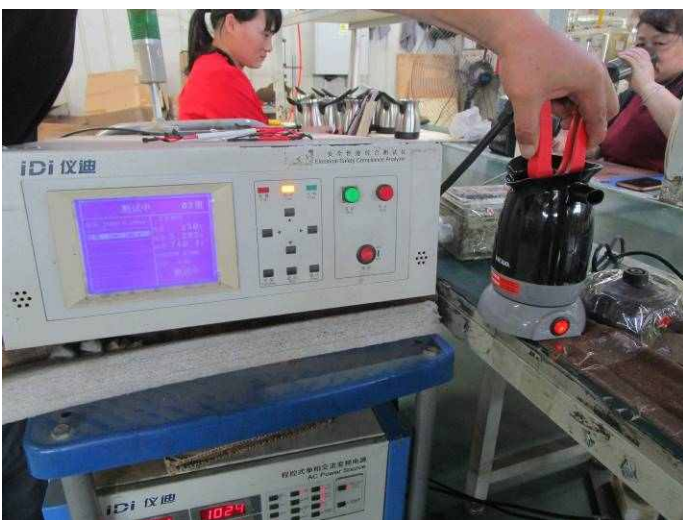
Hi-pot and Earth continuity test
