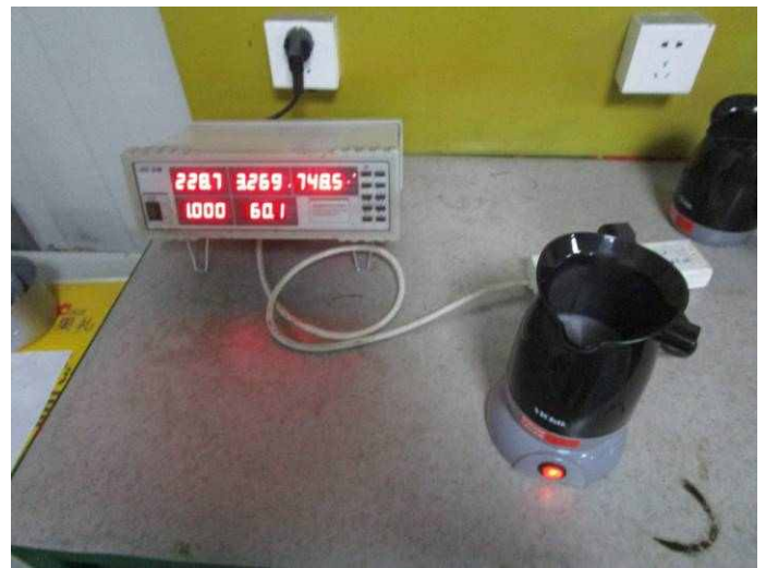
Power Consumption test with 230V
