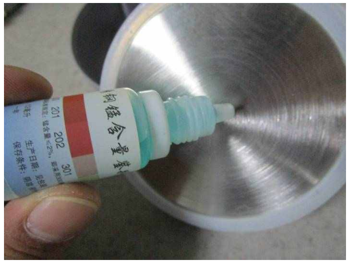
Stainless Steel material test
